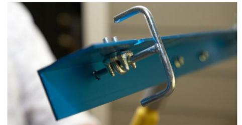
Gauge rakes are used to measure the product depth and help spread the material quickly.
