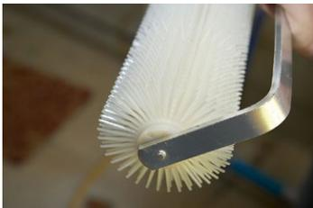
Porcupine rollers are an excellent tool to use in between bucket pours to break the surface tension of the product.
