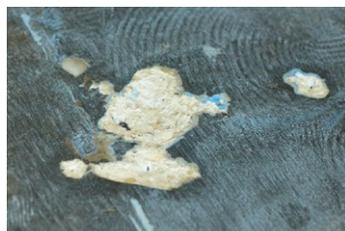
The depth of the dents and imperfections in the substrate can be seen more clearly just after the primer has been applied.
