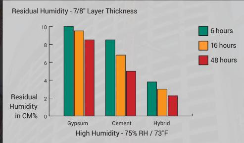
Drying speed based on AP Rapid Plus at 7/8". AP Rapid Plus may be poured at a thickness of 1/2" up to 3" with the Renotex® 3D System. Consult with your Schönox representative for more information.
