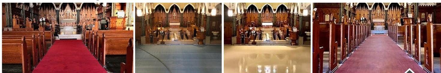
From red carpet over old, poorly adhered VAT tiles to new LVT tiles on a floating construction formed by Schönox AP Rapid Plus over Renotex® 3D.
